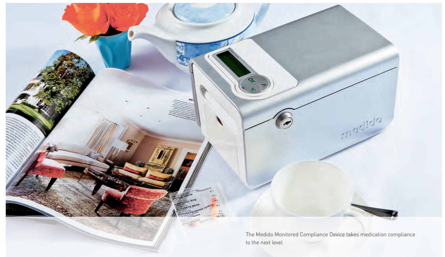
If a person fails to eject their medication sachet within a nominated period of time the device alerts a care giver for follow up
